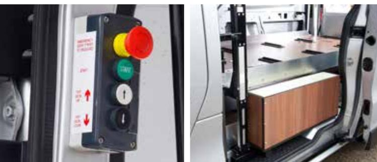
**Engineered for efficient operations**, the smart design of the Surelift has capacity for four stretchers or coffins courtesy of a motorised, dual height deck area.
